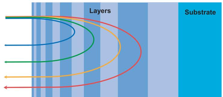
**Figure 1-** In a chirped mirror, the deeper penetration of longer wavelengths components within the incoming ultrashort pulse into the dielectric coating layers produces a negative GVD.
