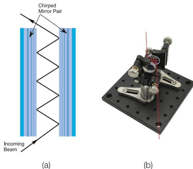
**Figure 5.** (a) Schematic diagram of a chirped mirror pair configuration (b) Chirped mirror pair mounted into Newport's clear edge mirror mounts U100-A2K to obtain the closest separation between two mirrors and allow for a large number of bounces.
