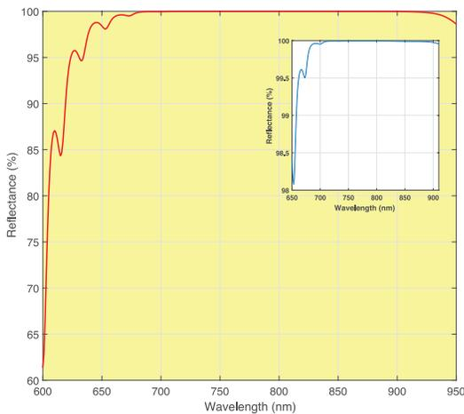
**Figure 2.** Theoretical reflectance as a function of wavelength for the Newport UF.40 ultrafast multi-layer dielectric coating chirped mirror. The dielectric coating design delivers reflectance that exceeds 99.9 % over the 700-900 nm range.
